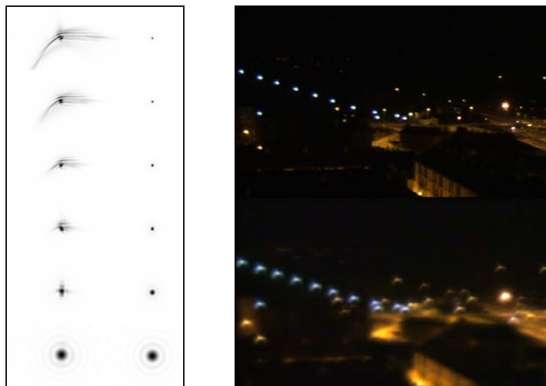
Figure 3. Left image: (Left column) The PSF of an actual eye for different pupil diameters, from 6 mm (top) to 1 mm (bottom) decreasing in steps of 1 mm. (Right column): the PSF of an ideal eye with no aberrations, for the same pupil sizes. Right image: (Top) An urban nightscape. (Bottom) The same nightscape as would be seen with the aberrated eye with a fully dilated pupil.
